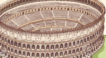
The interior of the Colosseum consists of six concentric and tiered walls that rise on a concrete oval surrounding the area of the arena. This framework of the entire structure can be compared to the reinforced concrete skeleton of modern buildings. It consists of arched walls made of blocks of
